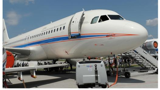
Ready for the first rolling tests with the DLR Airbus A320 research aircraft, ATRA (Advanced Testing and Research Aircraft). Aircraft fitted with this nose wheel will be able to approach their apron locations travelling in both forward and reverse directions, as well as taxi to their take-off positions without needing towing vehicles or using their main engines.
