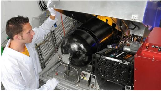
A fuel cell system delivers electrical energy capable of powering the nose wheel of a 70-ton aircraft.
