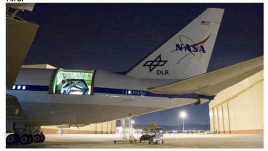
SOFIA during test observations of the night sky in March 2008. The opening in the fuselage of the converted Boeing 747SP provides a glimpse of the 2.5-metre infrared telescope, built in Germany.
