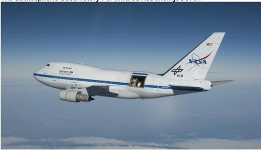
The Stratospheric Observatory For Infrared Astronomy, SOFIA, during its first test flight with its telescope exposed, on 13 July 2010. The German-built 2.5-metre infrared telescope is visible through the opening in the aircraft.
