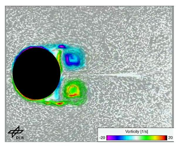
What happens when a cylinder is placed in flowing water? What vortices form behind a knife-edge or on an aerofoil? Footage captured by the Göttingen aeronautics pioneer Ludwig Prandtl 80 years ago, when fluid mechanics research was still in its infancy, provides the answers to these questions. The quality of these early films was so good that DLR researchers were able to evaluate them using modern measurement techniques, leading to worldwide acclaim and the award of an international prize.
