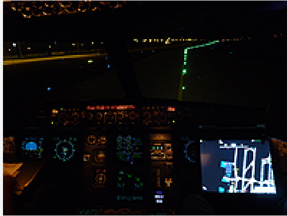
Cockpit of ATRA, showing the taxi guidance display developed by Diehl Aerospace GmbH
