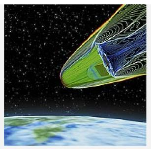
Numerical flow simulation on the EXPERT Earth atmosphere re-entry vehicle
