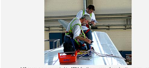
140 sensors are connected to ATRA for the purpose of acceleration measurement
