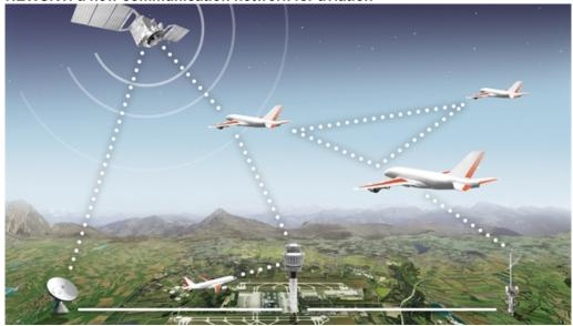
In the NEWSKY project, a communication network is to be created which meets the requirements of the aviation industry of the future. Here, the data streams must, above all, flow reliably between the aircraft and the ground, and this must happen both in remote regions over the oceans and the poles as well as in crowded conurbations. Supplementary information means that NEWSKY can sustainably improve safety standards in aviation and also reduce environmental impact through optimised flight paths.
