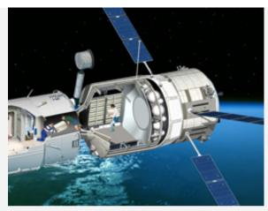
Docked with the ISS - cutaway view of the inside of the ATV
