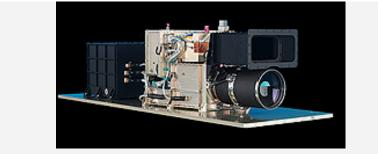
Close-up view of the High Resolution Stereo Camera (HRSC)
