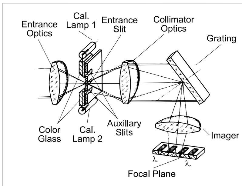
Fig. 4: Principle of the Imaging Spectrometer – Internal Calibration
