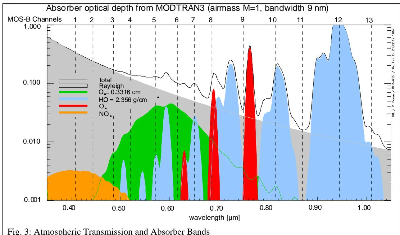
Fig. 3: Atmospheric Transmission and Absorber Bands
