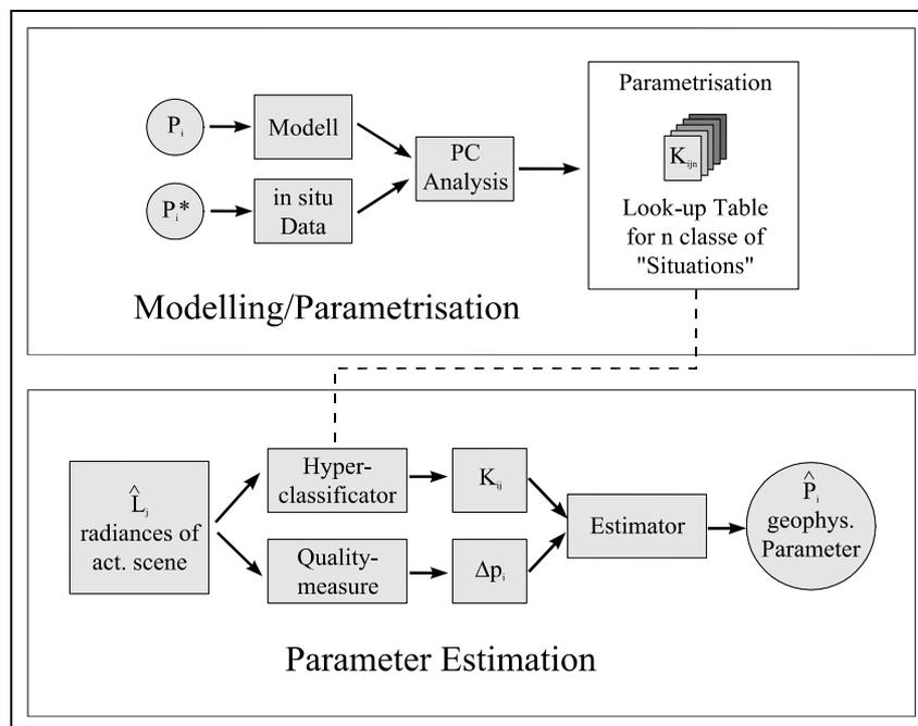
Fig. 9: Scheme of PCI Algorithm
