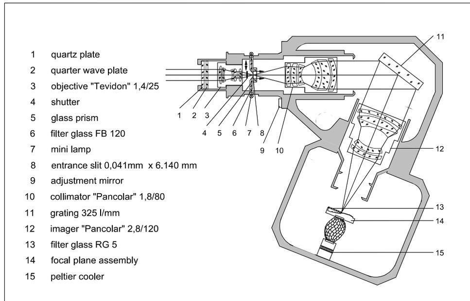
Fig. 2: Opto-mechanical Design Scheme of Block MOS-B
