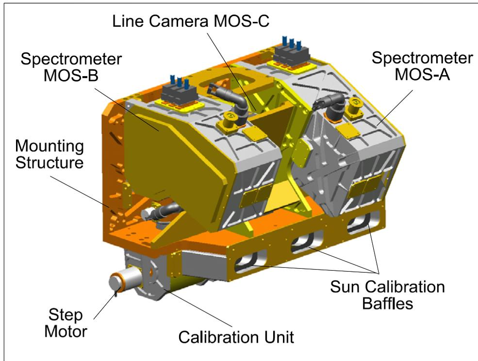
Fig. 1: Modular Optoelectronic Scanner MOS-IRS
