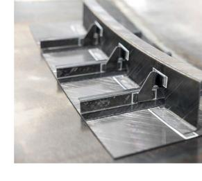
State of the art for the consolidation of large-area components made of continuous fibre-reinforced high-temperature thermoplastics, such as CF-PAEK, is the autoclave consolidation process. Through an optimised process setup and tailored process control, it is possible to achieve complete consolidation using only temperature and vacuum pressure. The use of self-heated
