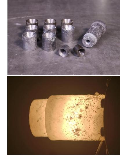
powdery phenolic resin. After the pyrolysis of the CFRP tubes and nozzle, the C/C preforms were machined, joined and siliconised. Firing tests of the thrusters in a vacuum chamber showed a high temperature resistance and a low abrasion of the nozzle throat diameter, determined by computertomography before and after the tests.
