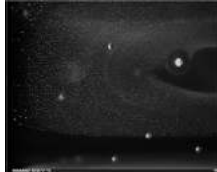
FIG. 1: Side view of a complex plasma containing microparticles (small white dots) and metallic spheres (larger white circles). The particles are illuminated from the left, which is why the spheres show a characteristic half moon. The cavity surrounding the sphere in the center right is caused by electric repulsion of the microparticles, while the large particle-free region in the right is due to plasma-specific effects. Field of view: 26 \times 36 mm 2 .
