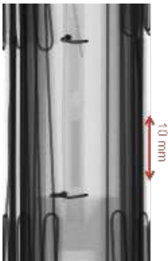
FIG. 1: X-ray image of the liquid sample (dark rod in the lower center) inside the furnace. No free surfaces or bubbles were observed in the sample. The heating wires of the two independently controlled heating zones can be seen as well.
