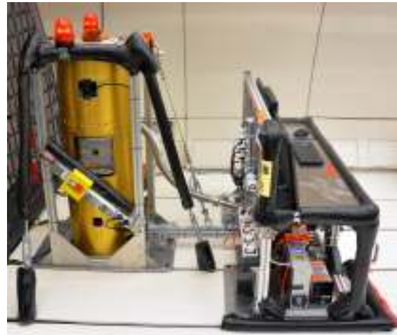
FIG. 1: The GOLD-ESL Experiment is shown in flight configuration onboard the Zero-G aircraft. On the left the rocket payload is fixed into a rack. On the right the experimenters rack containing auxiliary equipment can be seen.
