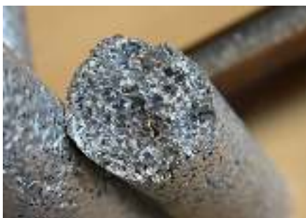
FIG. 1: Syntactic Al–Aerogel foams after dismantling of the steel tube.
