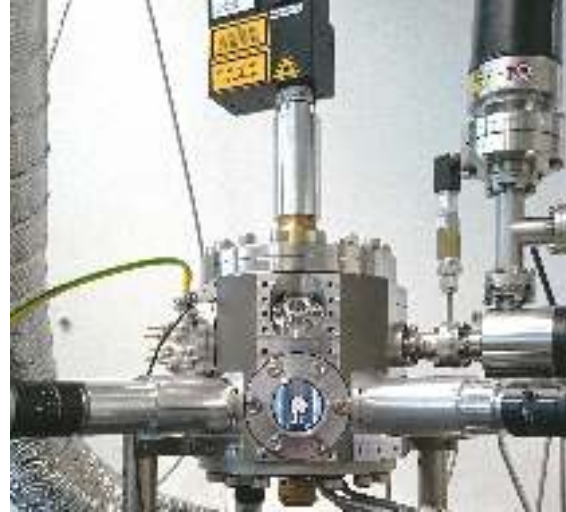
FIG. 1: The assembled Hybrid ADL-ESL Levitator in the lab
