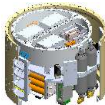
FIG. 1: CAD model of DEMIX with structure in sectional view (top: furnaces in process chambers (transparent), left: umbilical, right: gas tanks, orange: battery packs, green: daq)
