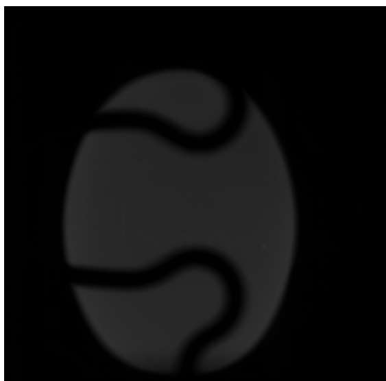
FIG. 1: Ni-base superalloy excited to surface oscillations by application of a heater pulse
