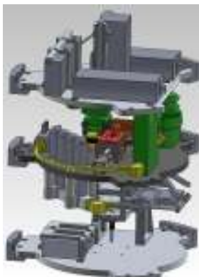
FIG. 1: CAD-drawing of the experimental module. The laser and detectors are mounted on the top panel, the gas agitation system and the sample cell on the middle panel. Below the middle panel a collimator feeds the light into fiber waveguides attached to the detectors on the top panel.
