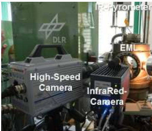
FIG. 1: Experimental setup to observe the solidification process simultaneously with a HSC and an IRC in front of an EML.
