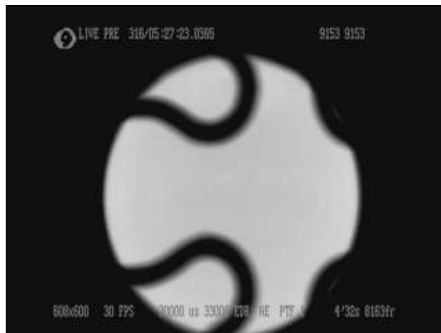
FIG. 2: Radial live video recording of the Zr sample during the facility checkout experiment (FCE). The dark patterns are wires of the cage, covering each sample.
