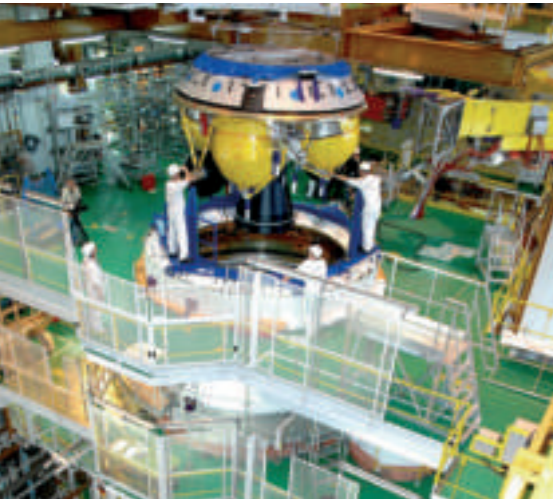
Bild links: Integration der EPS-V Oberstufe Picture left: Integration of the EPS-V upper stage
