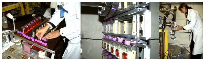
Exposure of human cells to energetic heavy ions at the "Grand Accélérateur des Ions Lourds" (GANIL) in Caen, France
