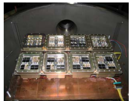
Biological samples accommodated for EXPOSE-R EST
