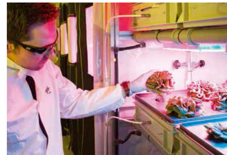
Multilevel growth system within the EDEN Lab incorporating water-cooled OSRAM LEDs and high-pressure aeroponics
