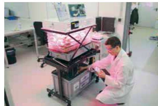
Dominik von Borell measuring the nutrient solution quality within the ORBITEC plant growth system
