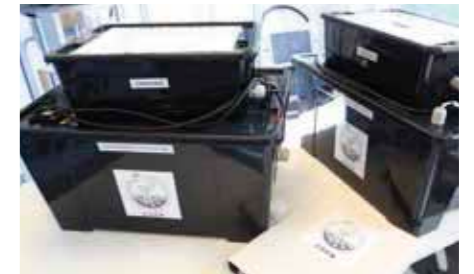
The EDEN- and the Schol_Lab Team built 10 low-cost plant growth boxes. The boxes can control light spectrum, relative humidity and temperature
