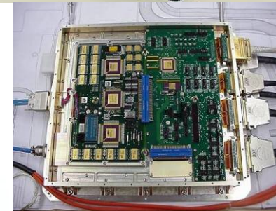
Cooler Drive Electronics
