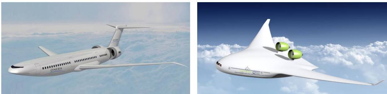
Figure 1: Left: A possible candidate for 2035 air transport: ONERAs NOVA concept with semi-buried engine (© ONERA, 2015). Right: Initial layout of a blended wing body anticipated for 2050 operation, equipped with generic UHBR engines mounted on pylons on the top of the centerbody (© University RomaTre, 2018).
