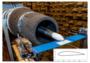
Figure 15: The baseline annular nozzle installed above the NACA4415 aerofoil on SOTON's Doak Laboratory Flight Jet Rig
