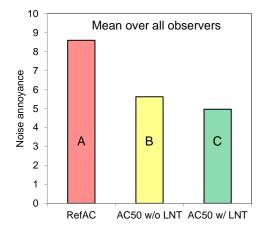
Figure 23: Main psychoacoustic experiment: Observed noise annoyance of the aircraft concepts (RefAC, and AC50 without and with LNT). Statistically significant differences (p < 0.05; pairwise comparisons with Bonferroni correction) are indicated by differing capital letters.
