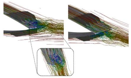
Figure 13: Near-wall instantaneous streamlines coloured with the magnitude of the total velocity on the suction and the pressure side.
