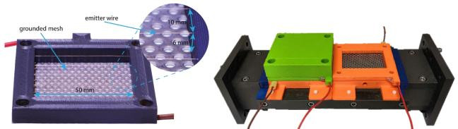
Figure 5: One cell plasma actuator (left) and two cell plasma liner prototype in a duct section
