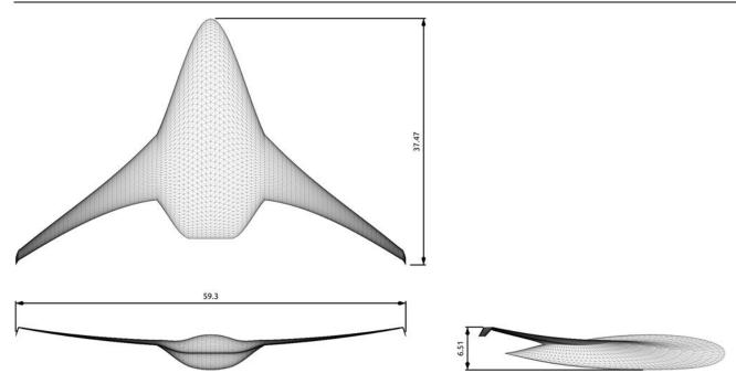
Figure 19: BOLT - optimized layout and main performance characteristics (©UNIROMA3, 2018)
