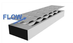
Figure 6: "Beam-array" liner concept
