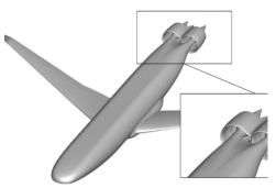
Figure 16: ONERAs NOVA NAUTILUS configuration
