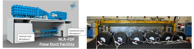
Figure 9: FDF test rig for high-speed testing of liners (left) and ZML-liner setup at FDF test section (right).
