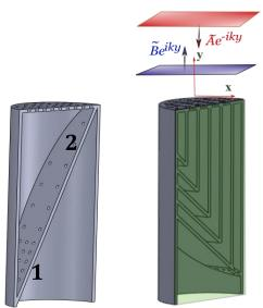
Figure 2: SOTON liner cell concepts for improved acoustic absorption. Left: Diagonal Septum Core ("Slanted Septum"), right: MultiFOCAL concept. (© SOTON 2019)
