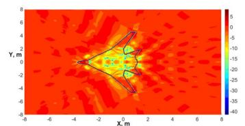
Figure 11: Shielding efficiency distribution (in dB) for a time-harmonic monopole source located above a planar polygonal screen of BWB-like shape.
