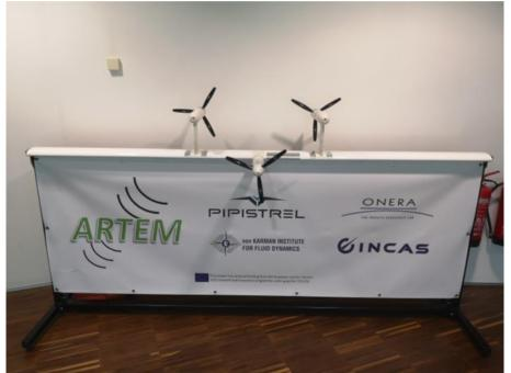
Figure 18: Wind tunnel model for DEP investigations: wing with 3 propellers mountable in pusher or tractor configuration
