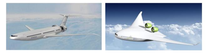
Figure 1: Left: A possible candidate for 2035 air transport: ONERAs NOVA concept with semi-buried engine (© ONERA, 2015). Right: Initial layout of a blended wing body anticipated for 2050 operation, equipped with generic UHBR engines mounted on pylons on the top of the centerbody (© University RomaTre, 2018).
