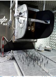
Figure 17: Landing gear model in AWB wind tunnel
