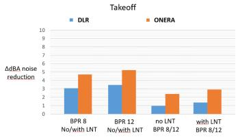
Figure 20: L<sub>A,max</sub> noise reduction between aircraft with and without LNT package (two to the left), and BPR8 and BPR12 configurations (two to the right) for takeoff configurations
