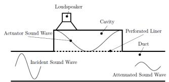
Figure 3: Zero Mass Flow concept by DLR. (© DLR 2019)
