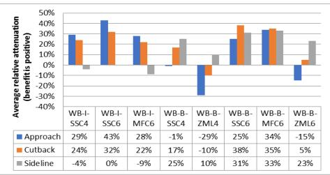
Figure 10: Relative benefit of the novel liner options for the Wide Body evaluator platform (Average in the frequency range of 500 Hz to 6400 Hz relative to datum for Bypass duct –B and -SSC4 for the inlet -I and 60 mm deep SDOF for the other, 60 mm deep novel inlet liner options –-SSC6 and –I-MFC6.
