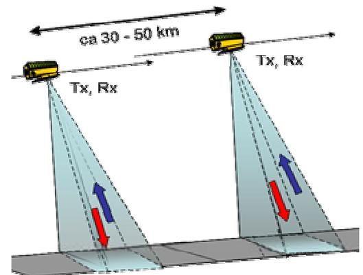
Figure 2. InSAR measurement configurations for TanDEM-X.
