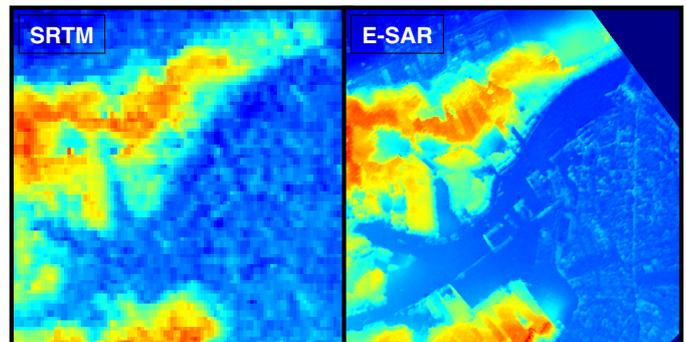
Figure 1. Comparison of DEM's with different DTED standards.
