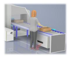
A laboratory model (technology readiness level  $\sim$  4) of the system was developed at the DLR Institute of Technical Physics, demonstrating the functionality of the technology.
