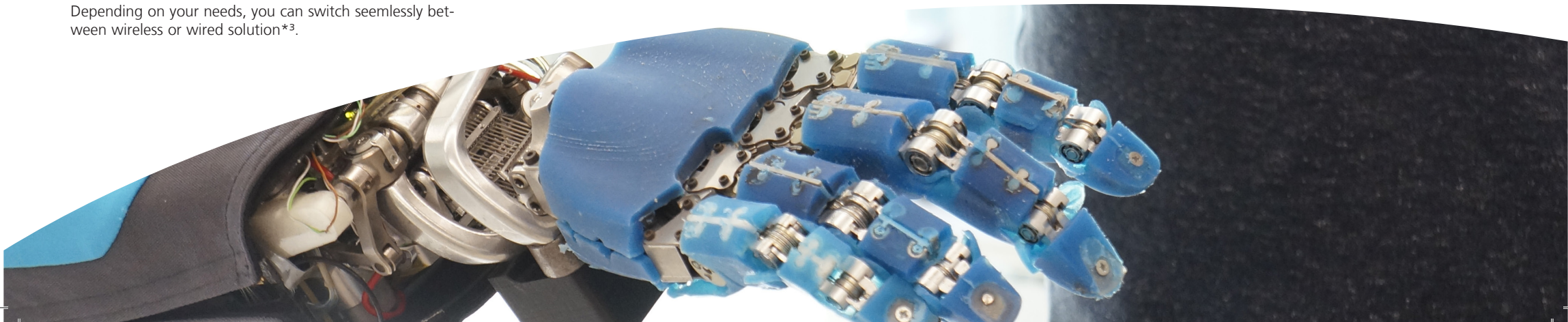
Accurate telemanipulation with the Kinfinity Glove on highly integrated Hand-Arm-System
