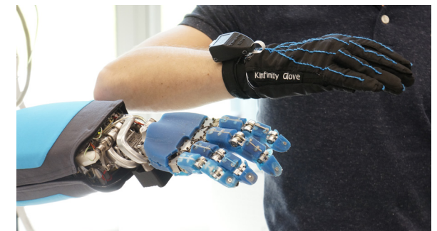
Accurate telemanipulation with the Kinfinity Glove on highly integrated Hand-Arm-System
