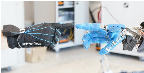
The Kinfinity Glove used in wireless mode
