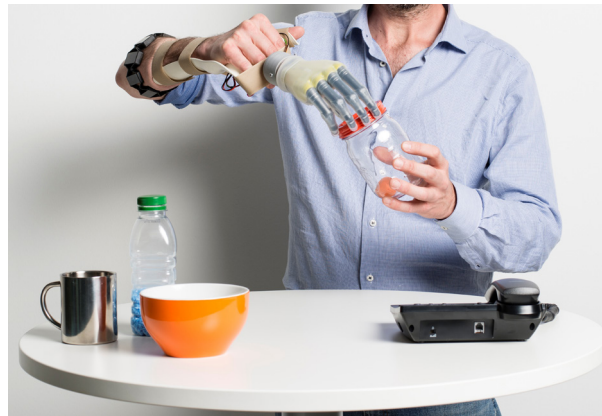
Testing prosthetic control with a non-amputated person
