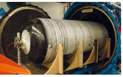
Ultralight CFRP high-pressure tank for hydrogen
