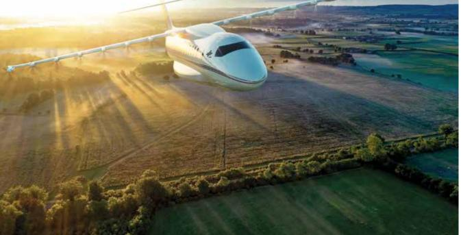
Electric flying enables new aircraft configurations, for example, distributed propellers at the leading edge
