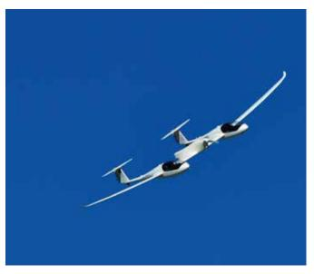
The Hy4 is the world's first four-seat passenger aircraft powered by a hydrogen fuel cell battery system. Its first flight was completed in 2016.
