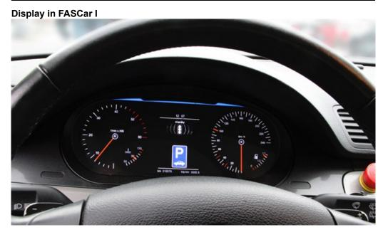
The parking sign on the vehicle's display signals an available parking place.
