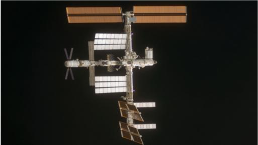
ATV Jules Verne docked with the International Space Station (ISS) in April 2008. This picture was taken from the Space Shuttle STS 124. The transporter, recognisable due to its X-shaped solar panels, can be seen on the left as an extension of the central axis of the ISS.
