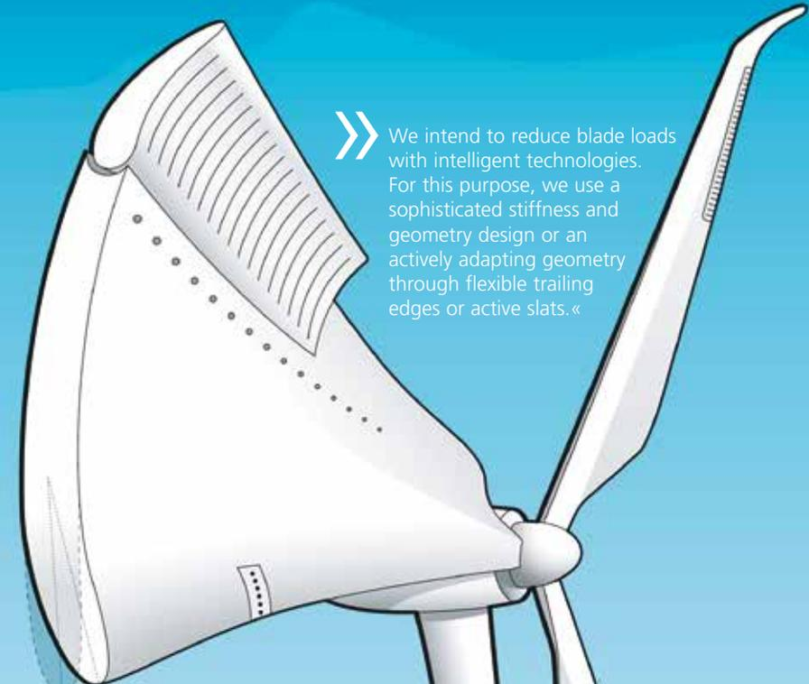
» We intend to reduce blade loads with intelligent technologies. For this purpose, we use a sophisticated stiffness and geometry design or an actively adapting geometry through flexible trailing edges or active slats.«
