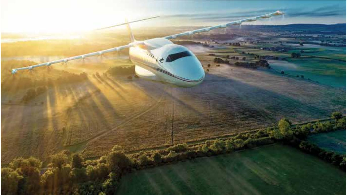
Electric flying enables new aircraft configurations, for example, distributed propellers at the leading edge
