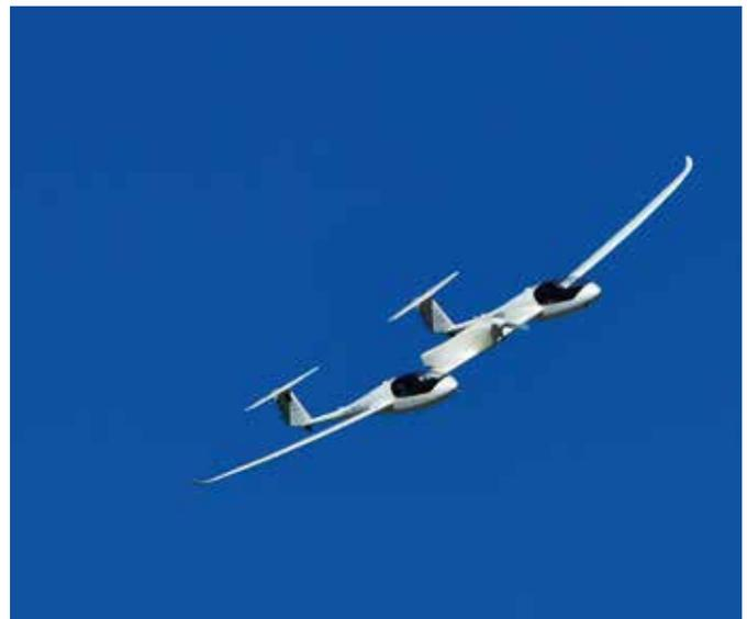
The Hy4 is the world's first four-seat passenger aircraft powered by a hydrogen fuel cell battery system. Its first flight was completed in 2016.
