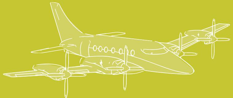
Battery-electric 19-seater transports synthetic fuel and a gas turbine as a reserve
