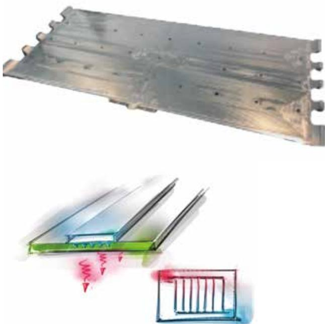
Multifunctional structure: supporting cooling plate for battery stacks
