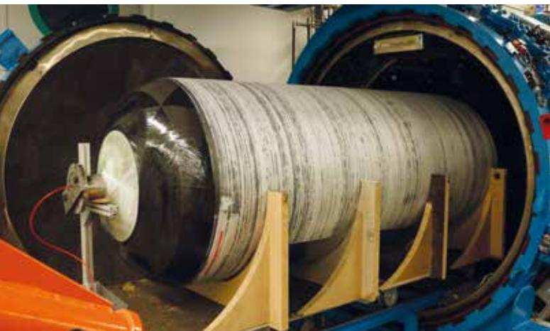
Ultralight CFRP high-pressure tank for hydrogen
