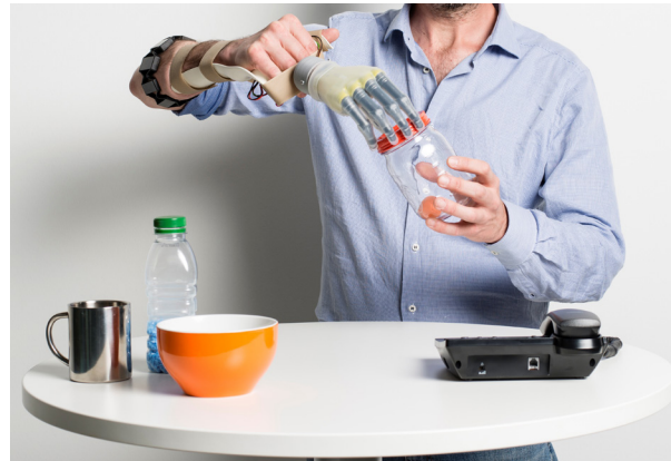
Testing prosthetic control with a non-amputated person
