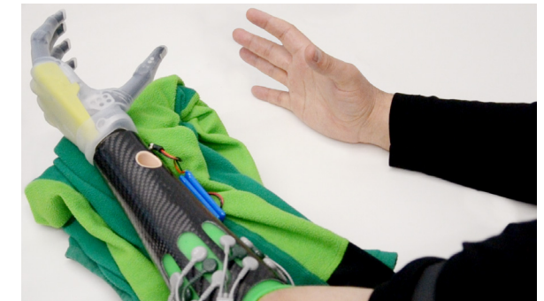
An amputated person uses the myocontrol system devised in the Prosthetic Laboratory
